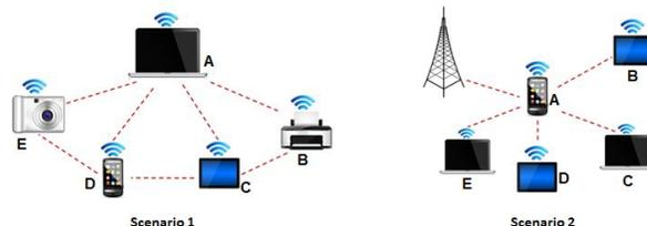
Figure 1. Typical Scenarios of Wi-Fi Direct Enabled D2D Networks.
